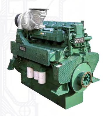
Maintenance is very easy, as supplementary equipment such as fuel injection pump, governor, water pump and turbocharger do not need any separate lubrication. The cylinder heads are individually divided by cylinder, and the engine has large inspection covers in crankcase and oil pan.
