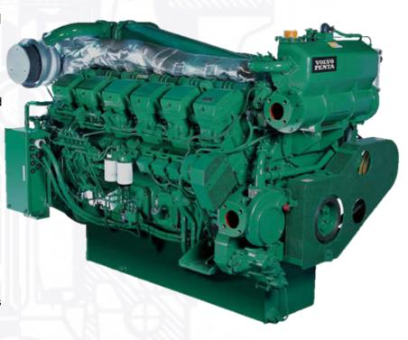
Maintenance is very easy, as supplementary equipment such as fuel injection pump, governor; water pump and turbocharger do not need any separate lubrication. The cylinder heads are individually divided by cylinder, and the engine has large inspection covers in crankcase and oil pan.
