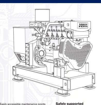
Easily accessible maintenance points and single side servicing contribute to the ease of servicing the engine. Liners of wet and replaceable type, inclined connecting rod caps and replaceable valve seats make even major maintenance possible to carry out on-board.
