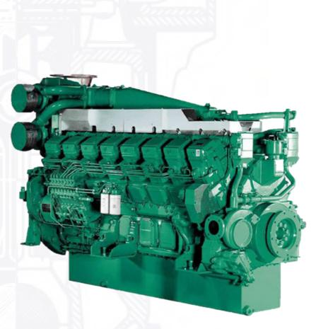
Maintenance is very easy, as supplementary equipment such as fuel injection pump, governor; water pump and turbocharger do not need any separate lubrication. The cylinder heads are individually divided by cylinder, and the engine has large inspection covers in crankcase and oil pan.
