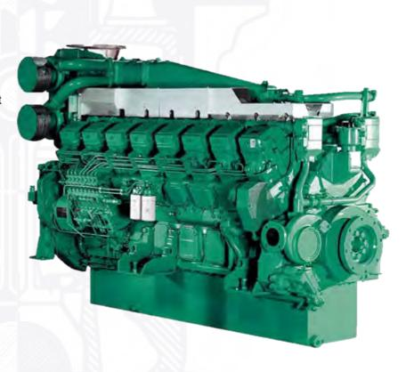
Maintenance is very easy, as supplementary equipment such as fuel injection pump, governor; water pump and turbocharger do not need any separate lubrication. The cylinder heads are individually divided by cylinder, and the engine has large inspection covers in crankcase and oil pan.
