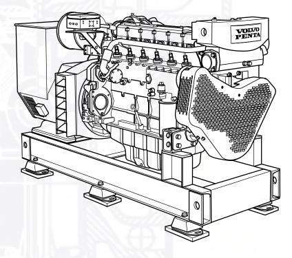
Easily accessible maintenance points and single side servicing contribute to the ease of servicing the engine. Liners of wet and replaceable type, inclined connecting rod caps and replaceable valve seats make even major maintenance possible to carry out on-board.
