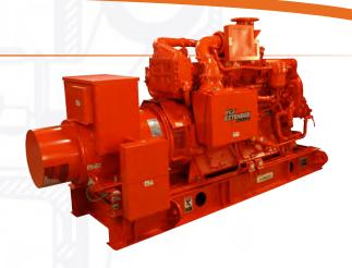
400/230, 3 phase, 12 wire Wye, 50 Hz. Temperature rise within NEMA 105° C for continuous duty, within NEMA 130° C for standby duty. Voltage regulation is  $\pm$  0.5%. All generators are rated at 0.8 power factor, are mounted on the engine flywheel housing, and have multiple steel disc flexible coupling drive.
